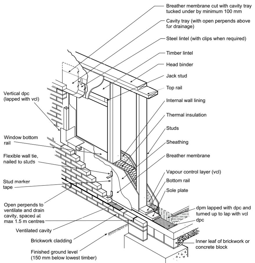
Figure 3: Externally sheathed timber frame wall with brick cladding
