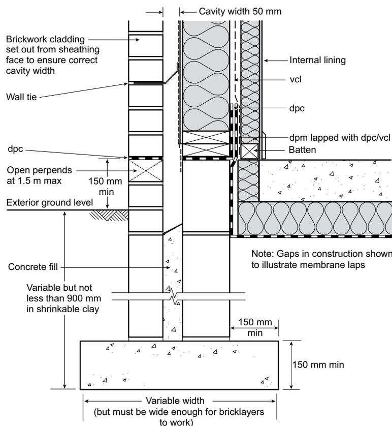
Figure 8: Strip foundation with masonry cladding
