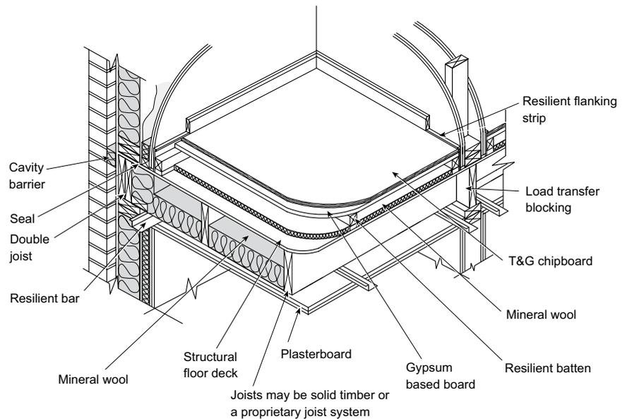
Figure 7: Party floor with solid timber joists
