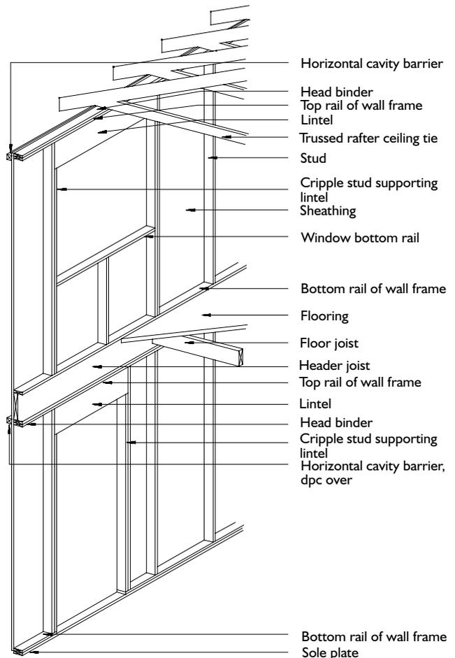
Figure 4: Typical external wall construction
