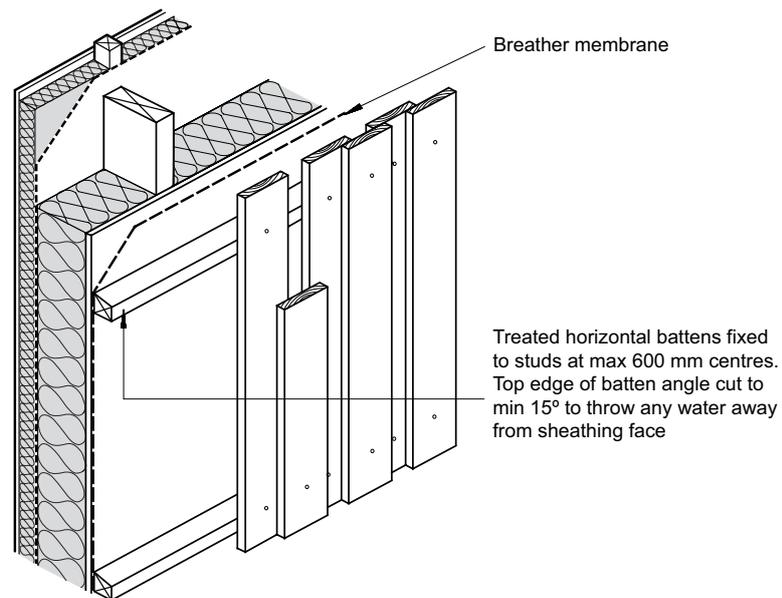
Figure 5: External wall with vertical board-on-board cladding
