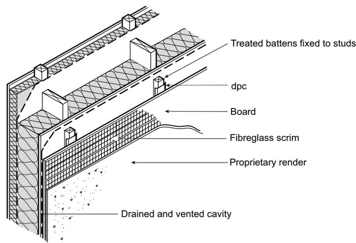
Figure 6: External wall with proprietary render system on backing board
