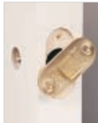
5. To reverse handing remove and turn latch 180° to re-fix
