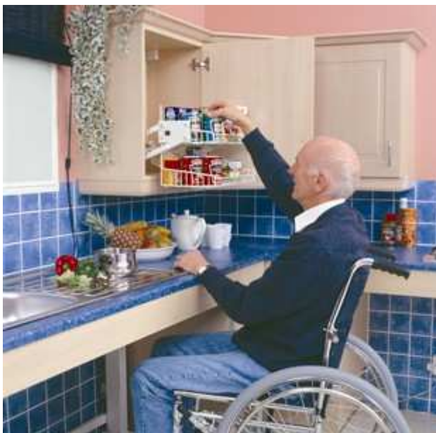
High level cupboard space designed for easy access for wheelchair users. Photo courtesy of Nicholls & Clarke
