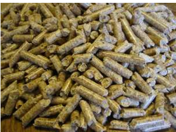
Wood pellets for use in a biomass boiler.
