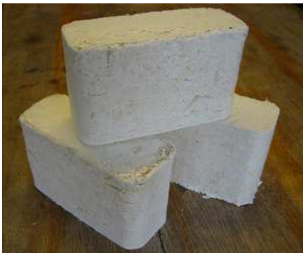
Wood briquettes for use in a biomass boiler.
